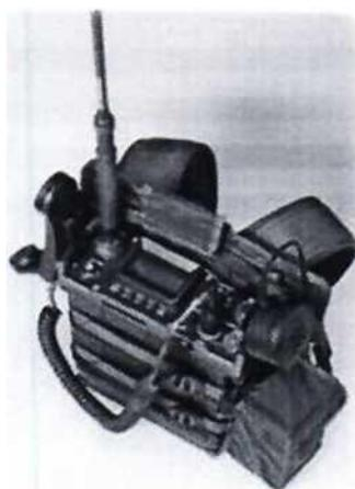
Backpack HF radio station (PRC - 6020) is intended for the organization of communication in a tactical control link. Frequency range is from 1.5 to 30 MHz
